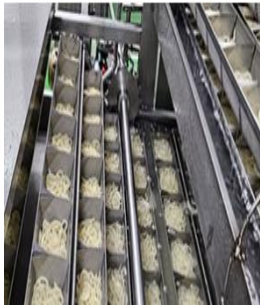
STEP 05 Cooling/immersion process
